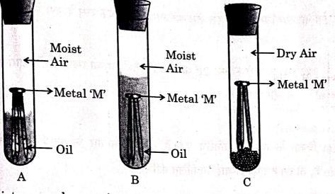
List your observations in each of the three cases A, B and C with reason, if the metal 'M' is generally protected against corrosion by the method of galvanisation.
